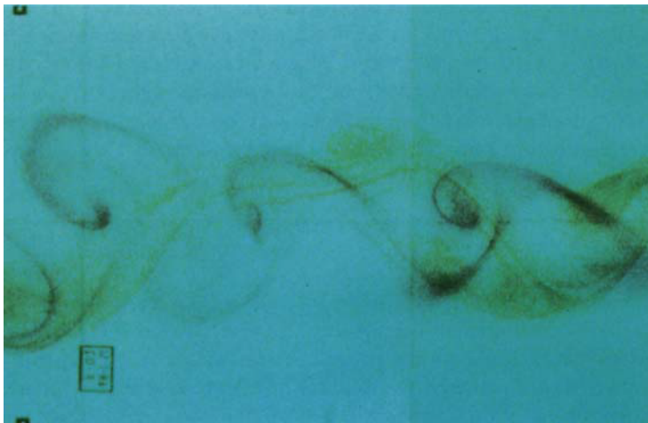
FIGURE 17. Vortex shedding at F = 0.2 behind \alpha = 1 ridge. Red dye injected at z/h = 0.5 ; yellow dye at z/h = 0.9 . The body is moving from right to left and is some way to the left of the left-hand margin. (Photograph reproduced from ciné film.)
